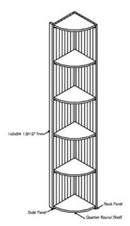
Step 3-Optional: (Attaching the  $1\times2\times84\frac{3}{6}$ " thm) Since the QR-G is not as deep as the other Apex Modular Racks, Apex has provided a 1x2x84  $\%_c$  long trim board as an optional piece when mounting the QR-7 to another modular rack. The trim board is used to fill in the gap between the QR-7 and the wall.
