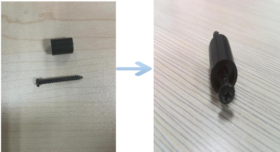
3. Towards the center right and left, just above the shelf, you will see holes on the interior of the cabinet. Insert the assembled screw and stopper into these holes and secure using a Philips head screwdriver.
