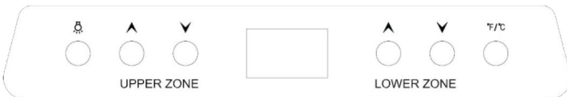
The upper zone temperature can be set between 45° and 54°F. The lower zone can be set between 54 ° and 64° F. Pressing the “UP” button on the control panel will increase the temperature by 1°F and pressing the “DOWN” button will lower it. Upon choosing your desired temperature, the display will flash the selected temperature setting for 5 seconds before reflecting the current internal cabinet temperature.
