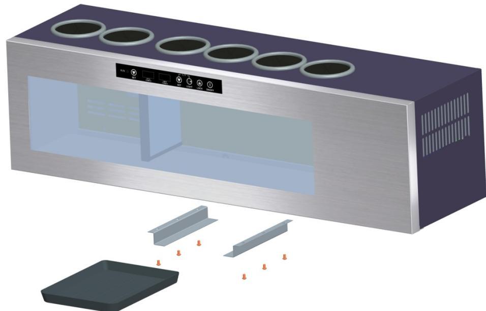
1. Affix the mount for the drip tray to the bottom of the cooler as shown in the diagram above.
