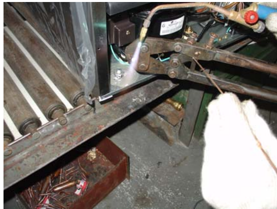
1-4-23、 Clamp the process tube and make it flat, and seal it after ensuring no leakage of the gas.
