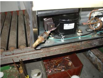
1-4-11、 Install the vacuumizing connector onto the process tube.
