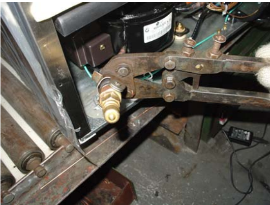
1-4-23、 Clamp the process tube and make it flat, and seal it after ensuring no leakage of the gas.
