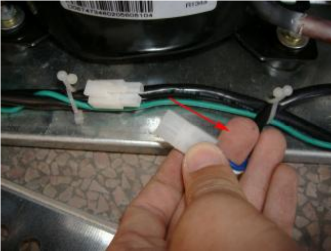
e. 更换新的风机 Replace the fan motor with a new one.
