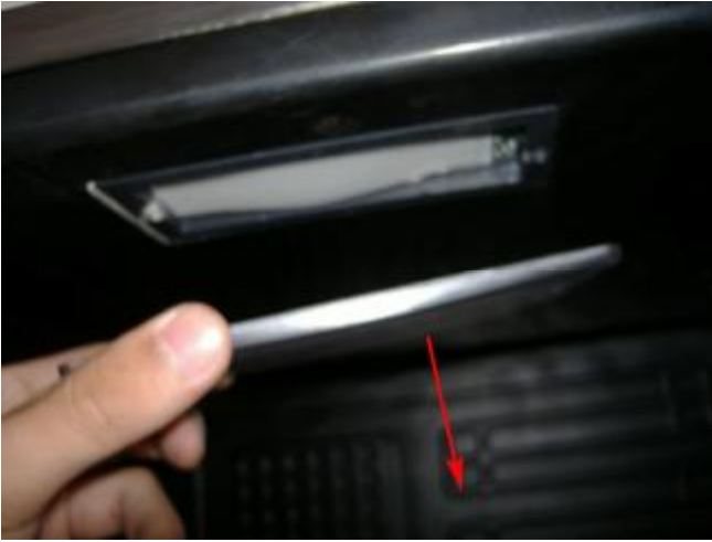
e.取出导光板 Take off the LED board.
