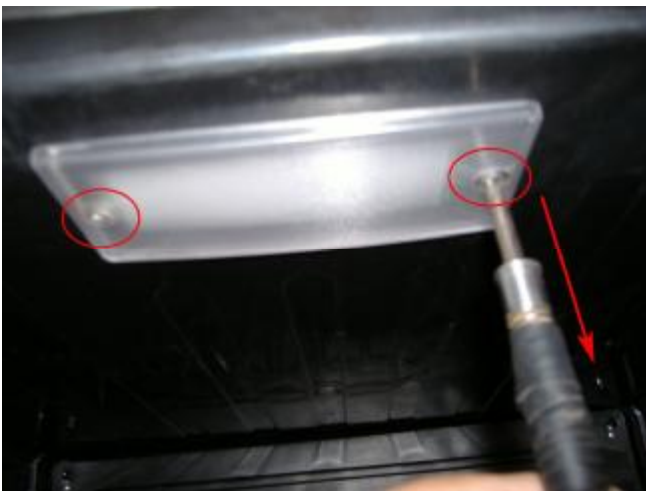
d.取下灯盖板 Remove the light cover.
