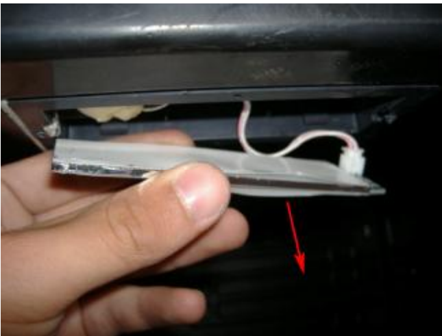
f.检查导光板上的接插件是否松动 Check if the connector on the LED board is loose.
