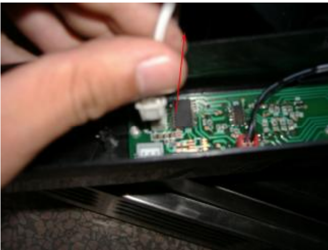
c.用剪子剪下接线柱图示部分 Cut the terminal according to the picture.
