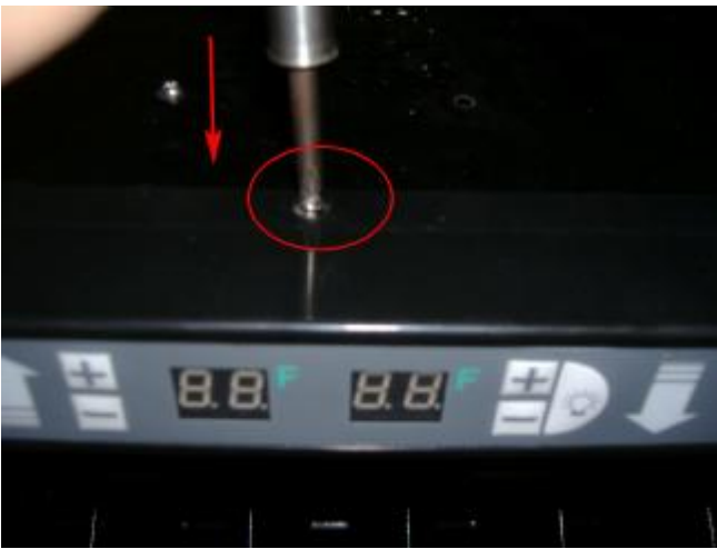
h. 安装温控罩壳 Fit in the plastic panel.
