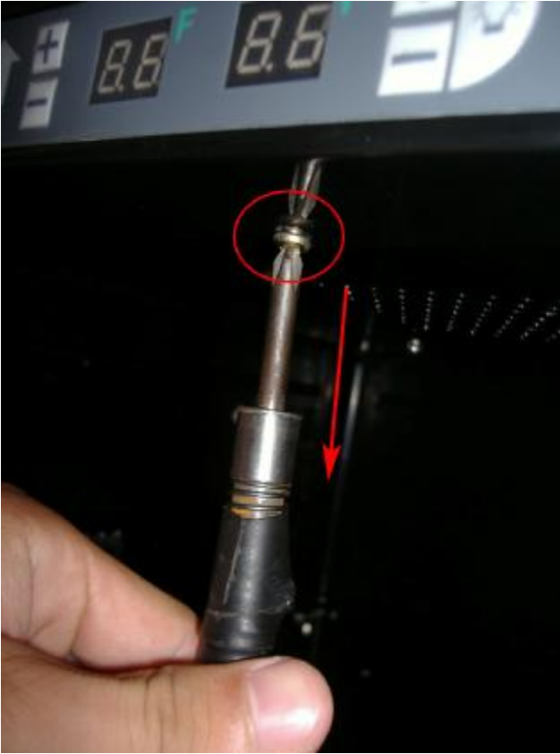
(2)取下数码温控罩壳 Take off the plastic panel.
