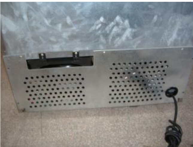
i.固定后封板 Fit in the back panel.
