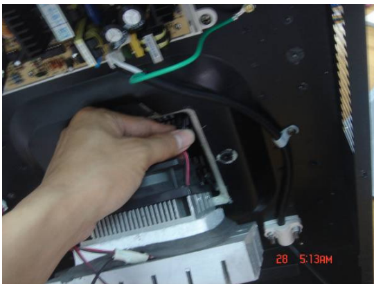
5) Pull cooling module away from the cabinet
