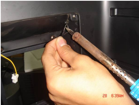
14) Heat the shrink tube
