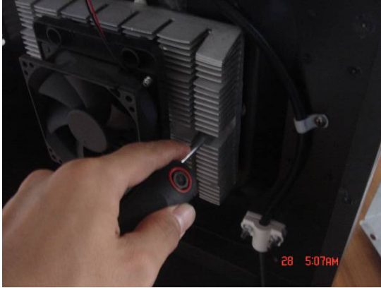
3) Move the cooling module
