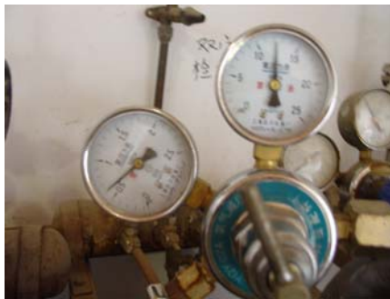
4-7-8、 Cover the welding point with towel that is soaked with soapsuds. If there is bubbles it means
