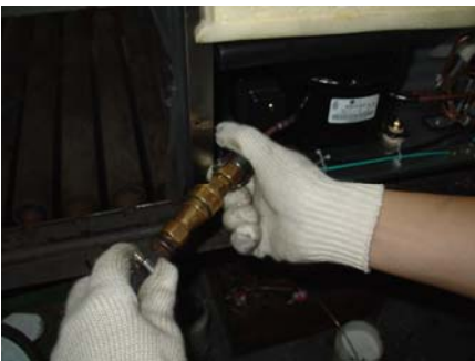
1-4-6-6、 Cover the welding point with towel that is soaked with soapsuds. If there is bubbles it means there is seam
