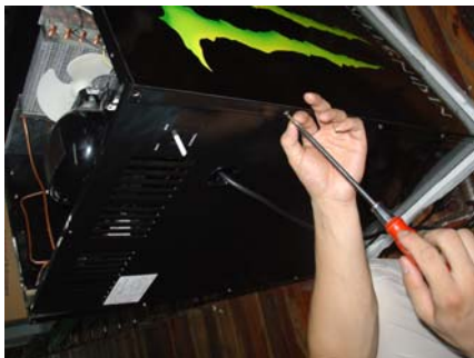
5-6、 Take off the fixing screws on the fan motor.
