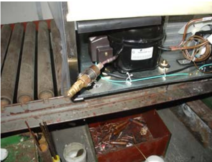
1-4-6-5、 Charge nitrogen. Charge 1Mpa the dried Nitrogen to the process tube
