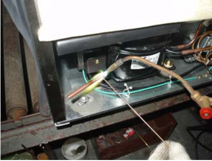
1-4-6-4、 Install the vacuumizing connector onto the process tube.
